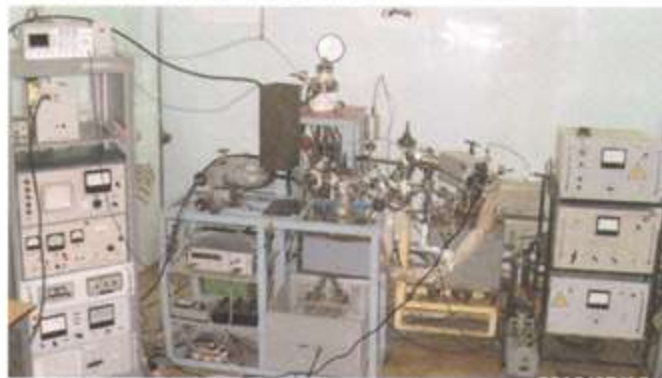
Figure: The experimental apparatus VIKa for studying thermal desorption of hydrogen isotopes from the materials
