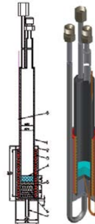
1-ampoule shell (12X18H10T), 2-cooling cover (12X18H10T), 3-heater (cable KTMС Ø4 mm), 4-sample (plumbic-lithium eutectic. (30 r), 5-thermo pairs, 6-thermal isolation, 7- nitrogen supply tube (Ø 6x1).
