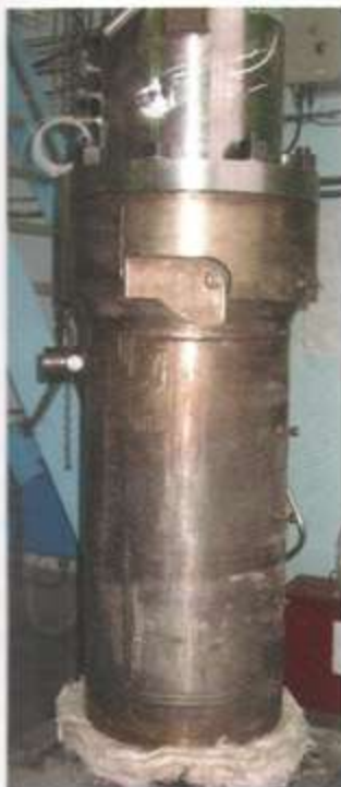
Fig. 2. Lower melt catcher in the unit for studying molten fuel cooling conditions in a pond with a sodium heat carrier
