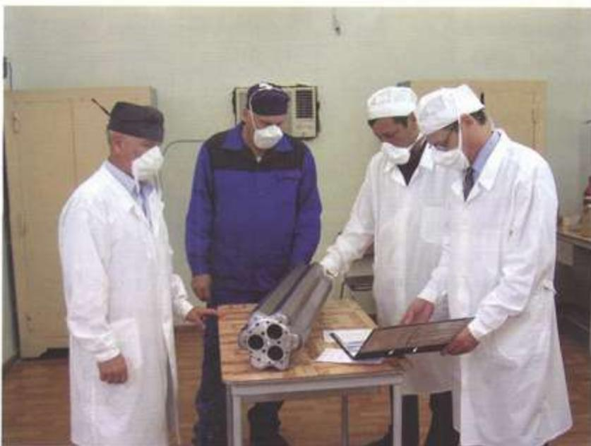
The first stage of the work includes testing of three fuel assemblies with lower-rich fuel in working reactor core region. To perform these tests we required a complex special facility made of beryllium and 28 hexagonal beryllium reflecting blocks.
