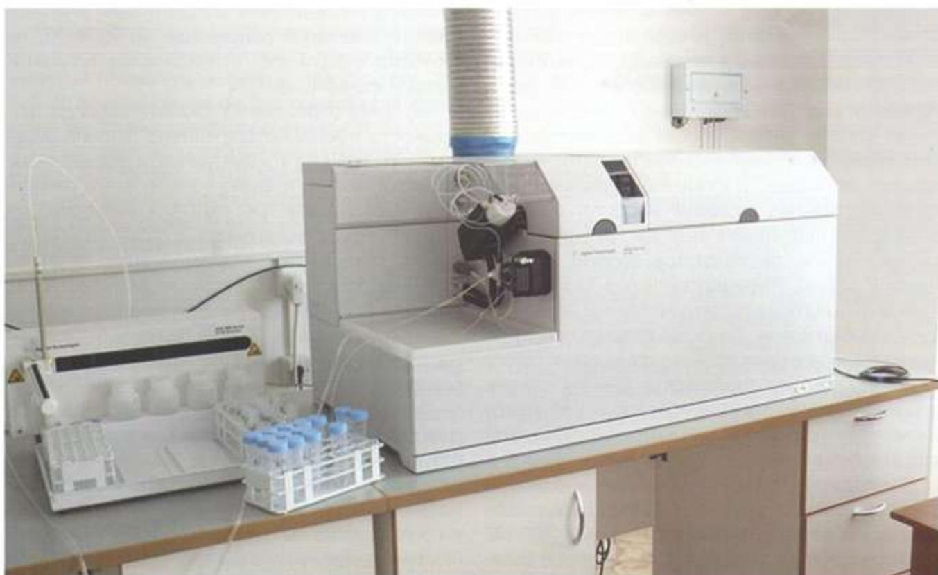
Fig. 1. Agilen-7500CX mass spectrometer with inductively coupled plasma
